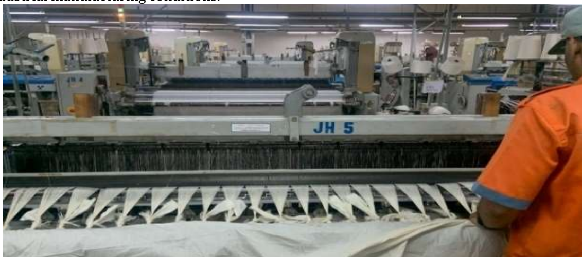
Figure 1. Toyoda Air-Jet Loom Used For The Experimental Weaving Trials Under Industrial Production Conditions
