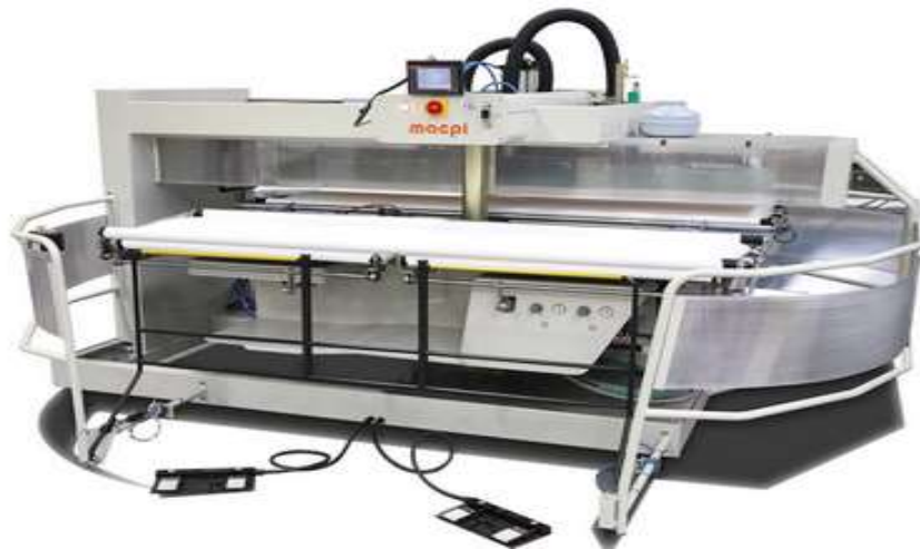
Gambar 3. Mesin Double Legger Merek Macpi Tipe 504-31-111 (Sumber : https://www.youtube.com/watch?app=desktop&v=0cYiWmHAsq4 )
